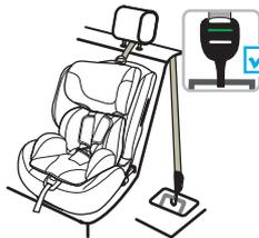
1. Take the top tether **18** out from the bottom of the car seat, adjust the Top Tether by pressing the Top Tether adjusting button **N**, and pass underneath the vehicle seat headrest.
