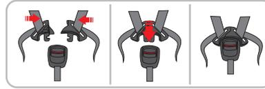
1. Put the right and left tongues of the buckle together, and insert into the harness buckle **07**, it is locked when a “CLICK” is heard. Pull the adjustment strap to tighten the shoulder straps **06**. Adjust the shoulder straps **06** so that the chest pads are close to the child’s chest. (Please refer 4-2 to check how to adjust the shoulder belt.)
