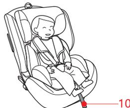
**Tighten:** Grasp the adjustment strap **10** with one hand and pull forward.
