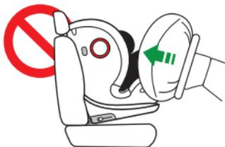
DO NOT install the car seat on a passenger seat with an active airbag.
