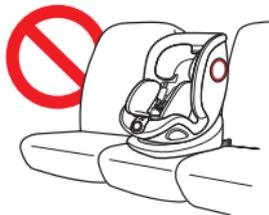
The car seat should not be installed in the vehicle middle seat.
