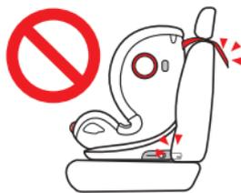
The top tether belt hook and ISOFIX should be suitable with the anchor points in the vehicle, otherwise it is very dangerous.
