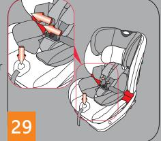
7.1.2. Relax the buckle: push down the red button on the buckle, the buckle tongue will jump out. Then put the harness at the both side of seat. (fig. 30)
