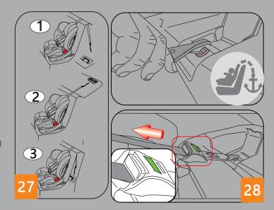
Finally check the child seat is fitted stable on the vehicle seat. If you find any movement you must tighten the top tether again until the child seat is tight enough.
