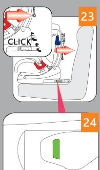
The correct locking will be confirmed when the "green colour" shows on the ISOFIX unlock button on both side (Fig 24).
